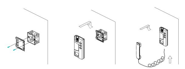
• Lock the wall wracket on the junction box with screws.
